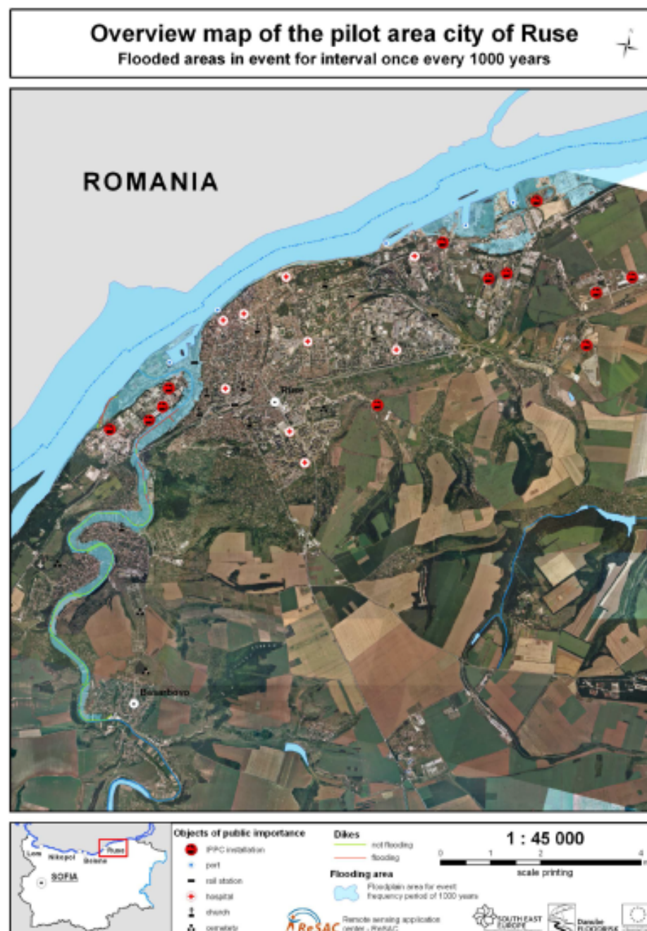
Fig. 4. Map of vulnerable territories and main elements of critical infrastructure for the city of Ruse and an imposed flood model with a periodicity of 1000 years, according to data from the National Institute of Hydrology and Hydrology
