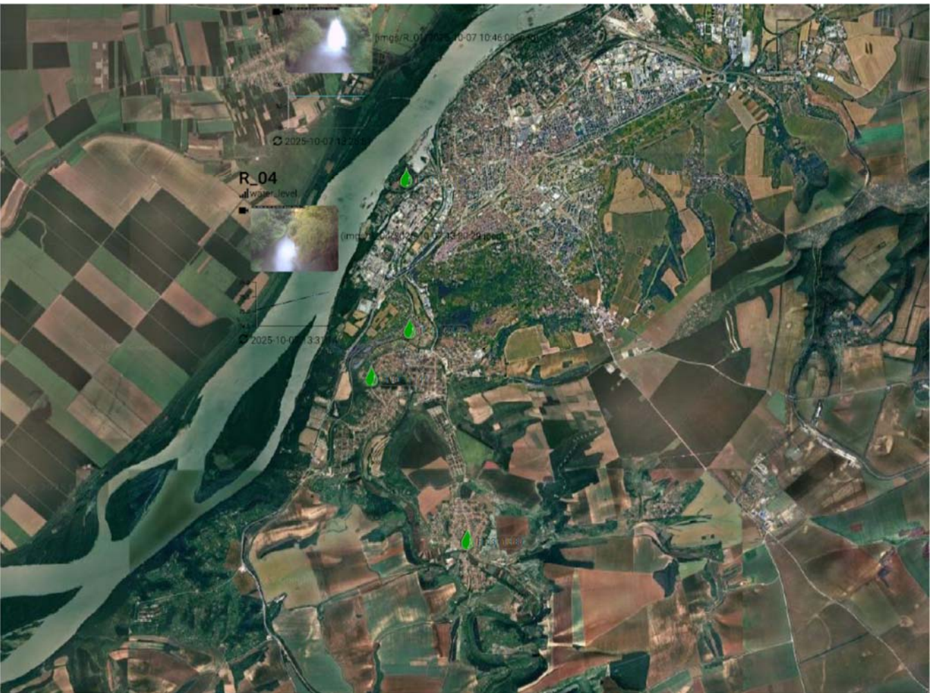
Fig. 1. Ruse City Laboratory - Pilot Site B - Rusenski Lom – B1 - current status - Ruse Municipality is building a sensor system (green drop sign) for ACWA early warning of flood hazards, including 24/7 monitoring of on-site data. Image source, Map data ©2025 Google. See website: https://ruse.acwa.app/mapWidget
